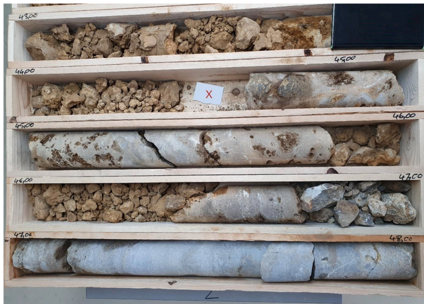
Fig. 4. Drill core section of core BK-6 at a depth of 43–48 m. Red X indicates a sample point in the karstified area of the core.
